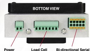
(12-24 VDC @ 6W) (Up to eight 350-ohm cells)
