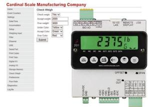
Checkweighing set-up is easy with the Web interface - set colors and weight limits remotely.
